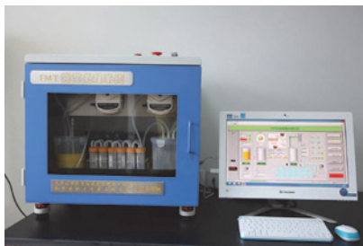
An automatic system called GenFMTer was used to isolate fecal microbiota from stool.
